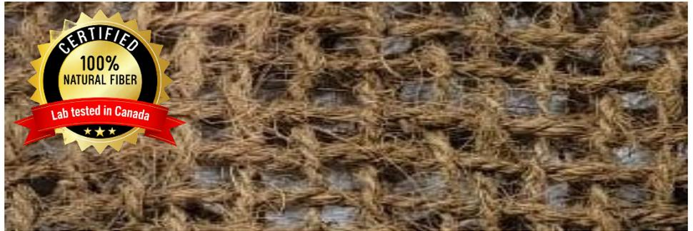
**NovaCoir 400 GSM** is a lightweight, biodegradable erosion control mat crafted from 100% natural coconut coir fibers. Designed for moderate environments and low-impact landscapes, it provides reliable surface protection while supporting ecological performance. With a density of 400 g/m<sup>2</sup>, it offers:
